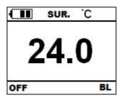
Surface temperature measurement mode
